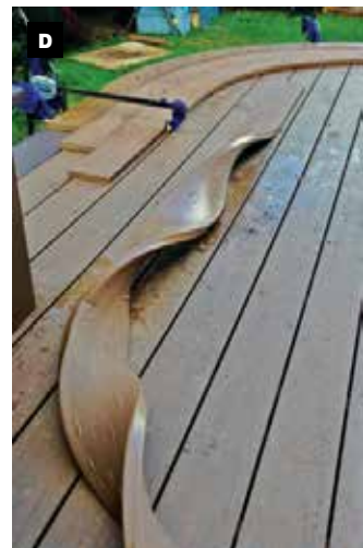
For custom bending, the author built forming tables equipped with adjustable clamps (A), as well as an insulated heat box (B) sized to accommodate Heatcon thermal blankets (C). Work carefully; excess heat will deform PVC and composite decking (D).
