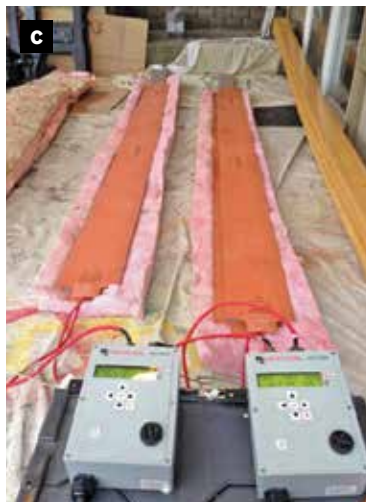
For custom bending, the author built forming tables equipped with adjustable clamps (A), as well as an insulated heat box (B) sized to accommodate Heatcon thermal blankets (C). Work carefully; excess heat will deform PVC and composite decking (D).
